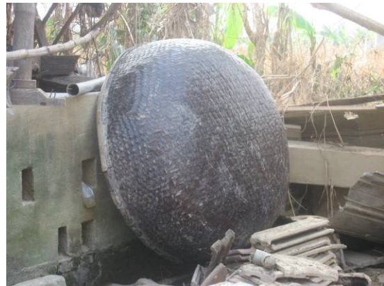
Measuring about 1.5 metres in diameter, these bamboo boats provide independent means of evacuation in flood situations for people in the Quang Ngai province. (Ewa Eriksson/International Federation)
