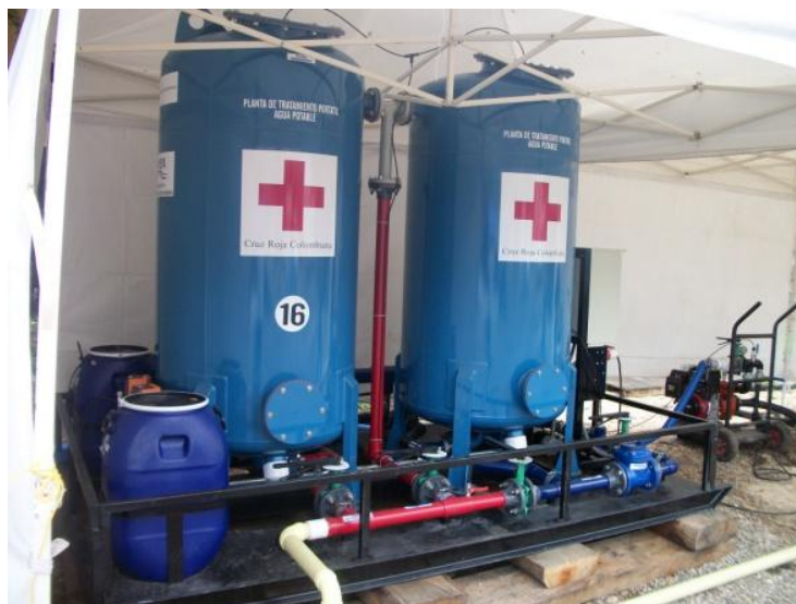
The Colombia Red Cross Society procured a new and more efficient water treatment plant that produces 2 litres of safe water per second. Source: CRCS
