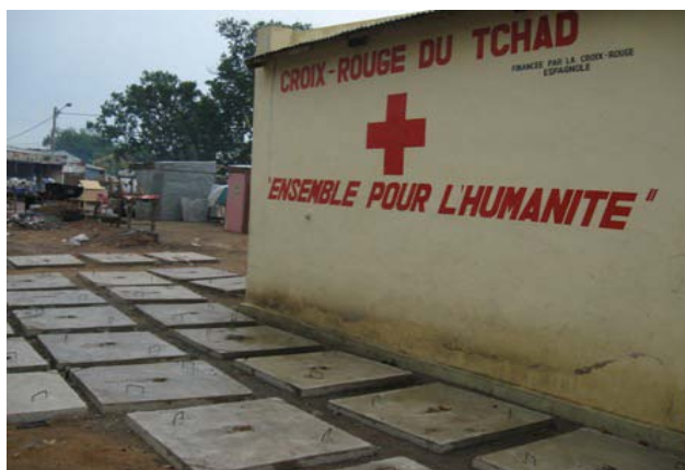
Sanitation platforms were built in the Red Cross of Chad branch in Bongor and distributed to vulnerable families in five affected districts. Photo: Mahamat Tahir Brahim/ Red Cross of Chad.
