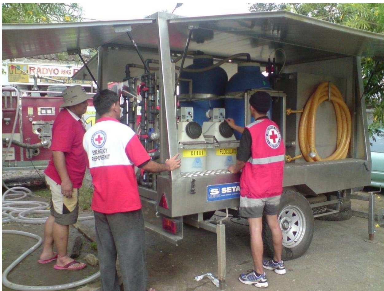
One of the two SETA water units providing clean and safe water services in the Aklan province that suffered badly from the wrath of typhoon Fengshen. (PNRC Disaster Management Services)
