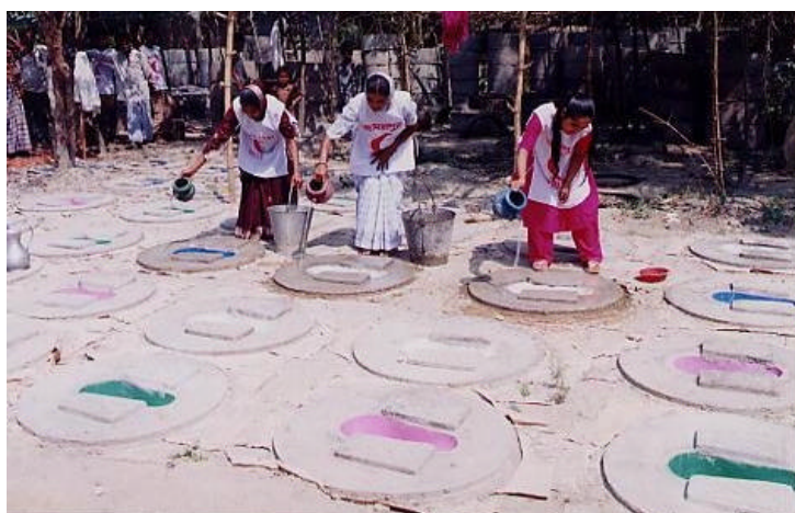
Female CBDP volunteers assisting in community based development program – production and installation of sanitary latrines
