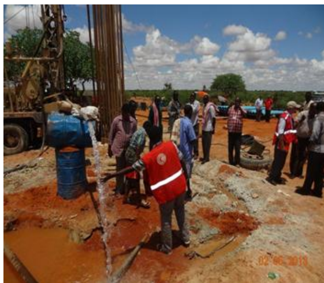
A pumping test being conducted at the new borehole in Laanmadow, Galkayo, Mudug region, Puntland. Photo/ SRCS.
