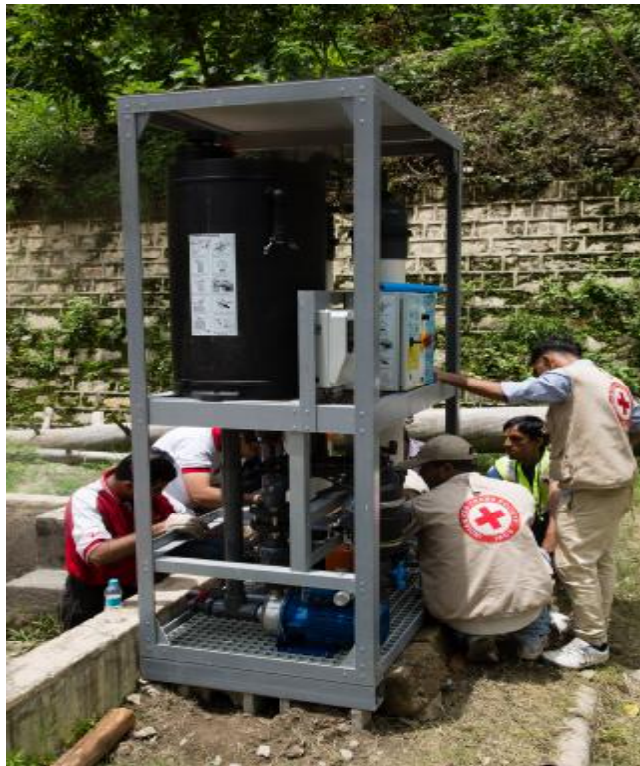
IRCS NDWRT members setting up NORIT water treatment unit in Uttarkashi. Photo: IFRC/Stephen Ryan
