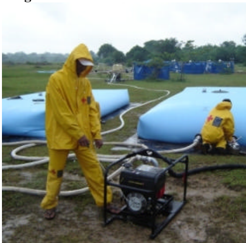
SLRCS are working with German Red Cross water specialists to produce up to 140,000 litres of clean drinking water every day.
