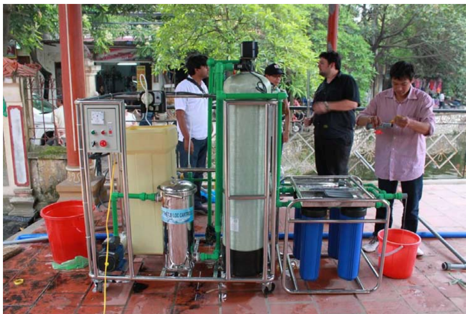
Testing of two locally manufactured water treatment units was carried out in Hanoi with technical support from IFRC and French Red Cross. Recommendations followed by further testing will be done in July to have these units operational by August 2011, prior to the annual typhoon season. (Photo: Vinay Sadavarte/IFRC)
