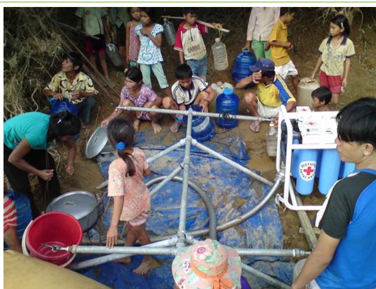
Recent water and sanitation training of VNRC staff and volunteers with IFRC support helped VNRC set up this water treatment unit independently and give families quick access to safe drinking water during the recent floods in Viet Nam. The IFRC plan supports capacity building in such activities which is imperative to enhancing national society service delivery and extending its reach to the wider community. (Photo: Tran Quang Tuan/VNRC)
