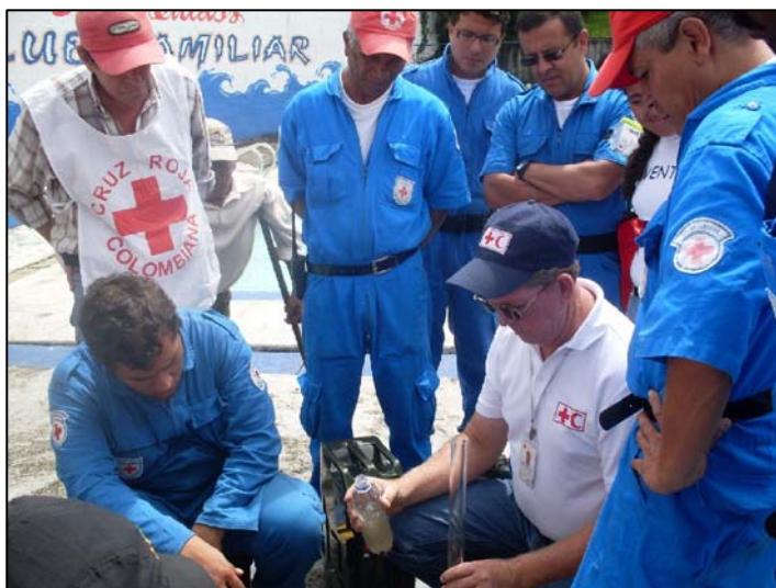
The RIT member showing CRCS volunteers how to analyze the water using chemicals. Source: International Federation
