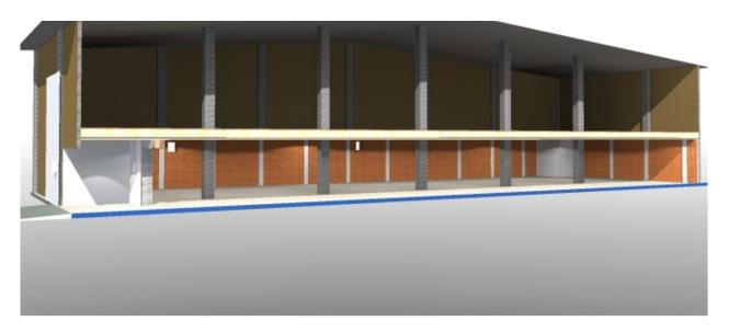
Architectural drawing of the green warehouse, showing double false ceiling and second walls. © ICRC, 2020
